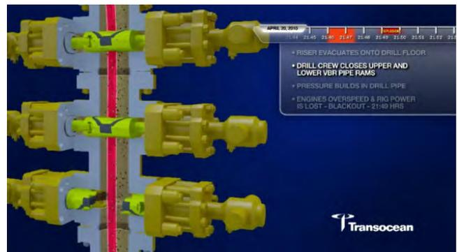
To see a fascinating video on how the Deepwater Horizon's Blow Out Preventer was supposed to work (and why it didn't), go to:
