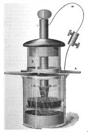
lower end, where it joins the body of the electrode, a piece of platinum foil reaching up a short distance, to increase the depository surface and prevent a powdery deposit on the
