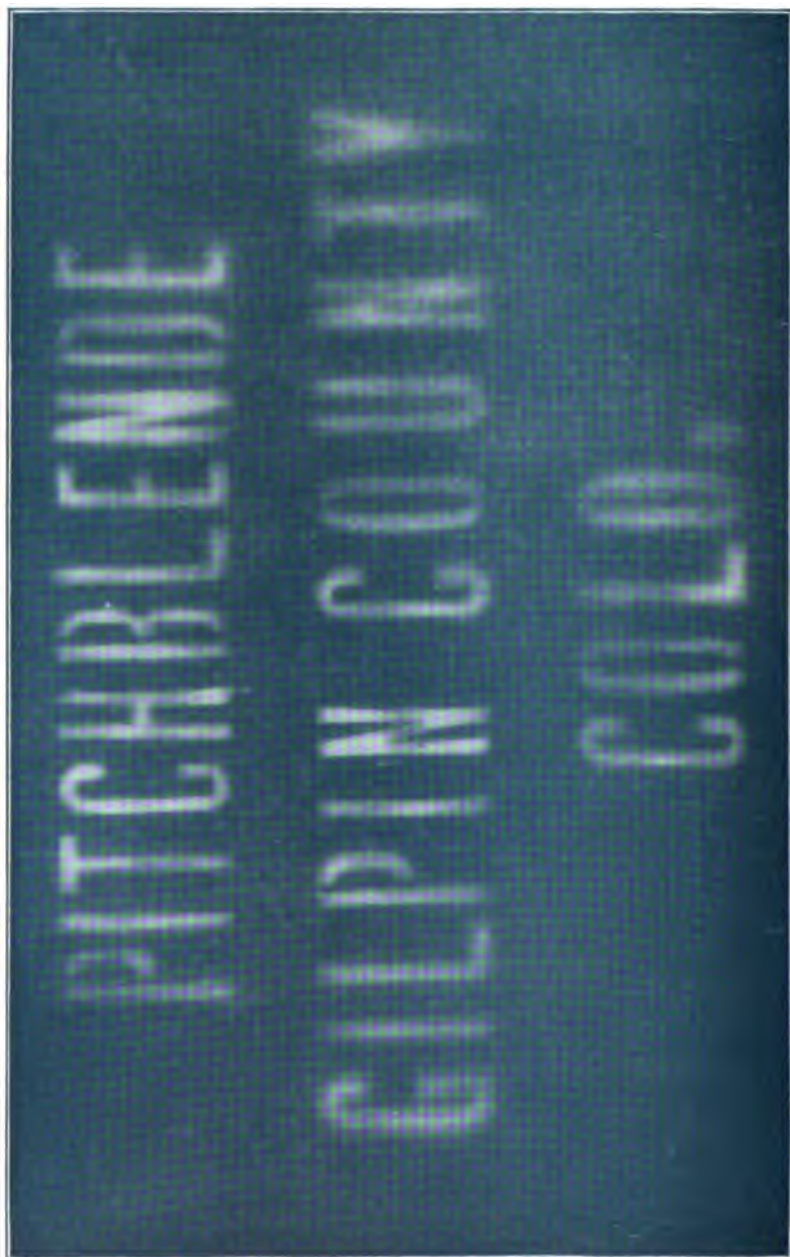
Radiograph taken with Pitchblende from Gilpin County, Colorado. The plate was exposed for two and a half days ; the distance between plate and mineral 0.25 to 0.50 centimeters.
