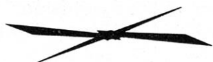
FIG. 7.—ILLUSTRATIVE OF THE TREND OF THE TUNGSTEN VEINS IN THE MAGNOLIA MINING DISTRICT. LENGTH OF LINE INDICATES RELATIVE IMPORTANCE OF VEINS.
