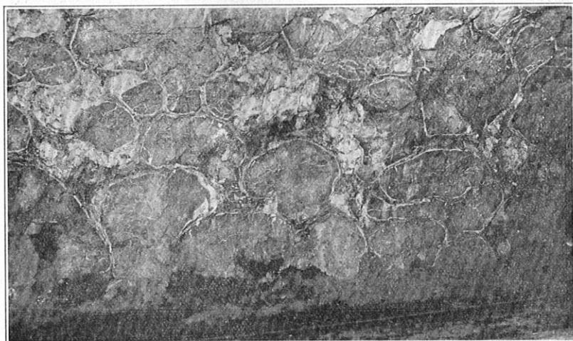
Pillow-lava formation in the andesite below the ore body at the 820-foot level of the Skouriotissa mine, Cyprus.
